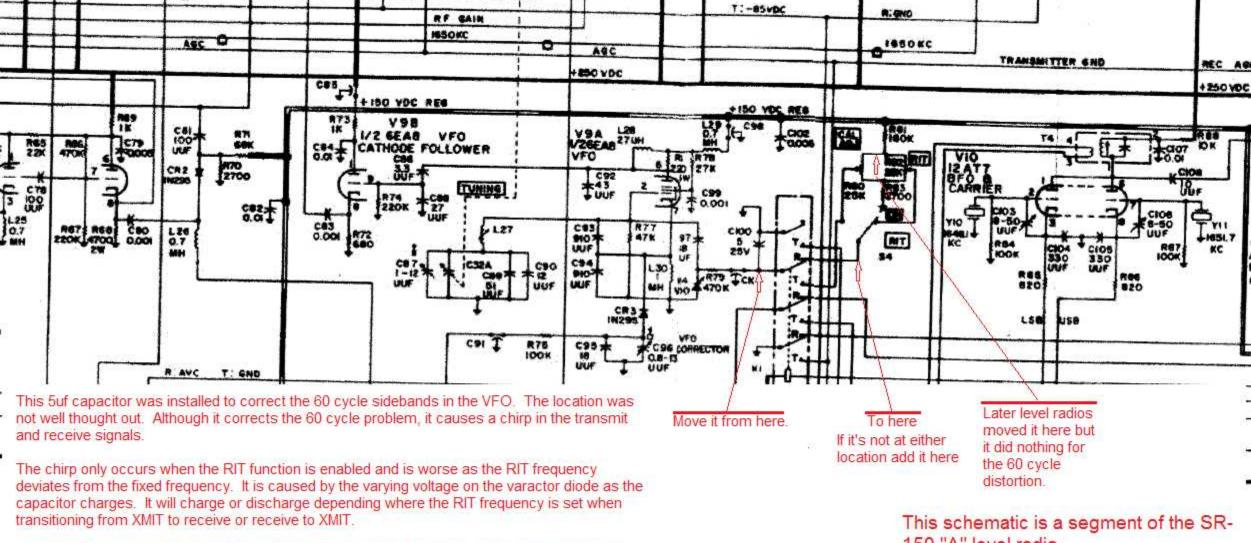
If you move the capacitor from where it is to the other side of the relay the chirp will only occur when you are in receive mode and when you flip the RIT switch. This is not a problem.
